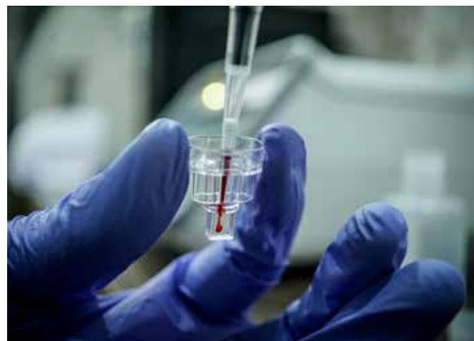
in 1 minute. Gazelle enables automated data acquisition and transmission of case-patient details to the malaria surveillance system resulting in real-time reporting. Targeted at cost of \$2 per test, Gazelle also supports multiplexing by testing for other diseases such as sickle cell disease, beta thalassemia, that often occur in the same area as malaria.
